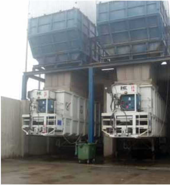
FIGURE 6 Two containers used at one of the seven existing waste transfer stations located in western Macedonia, Greece. The containers, once filled, are emptied in a sanitary landfill, washed, and brought back to the station. The pioneer integrated waste management project operating successfully since 1998 with the collaboration of four neighbouring prefectures, covers all stages starting from collection, re-transfer, sorting, recycling & manufacturing, sanitary landfill and special waste treatment.
