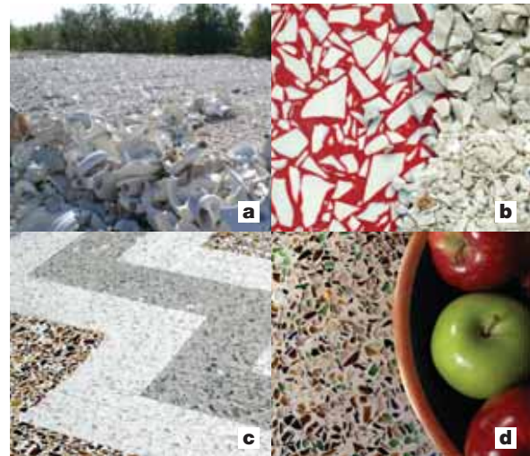
FIGURE 14 Starting from broken porcelain items (tubs, sinks toilets) and glass as raw materials (a) these may be transformed to terrazzo surfaces (b) that can be used as durable floors, kitchen or bathroom counters (c), (d) (case from USA).
