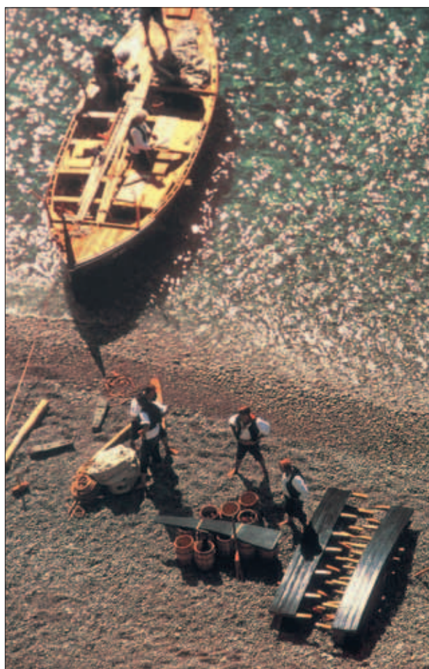
The "gaeta" turns from sailboat to finishing boat upon removal of the upper sideboard, beach of Palagruza (Croatia). The gaeta has a unique naval architecture combining two boats in one
